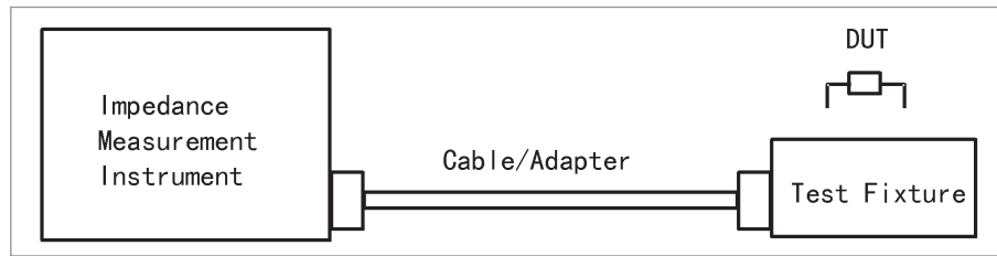
System configuration for impedance measurement
